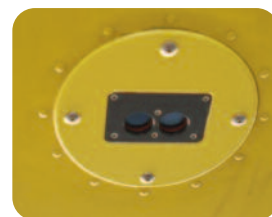
Laser module mounted in aircraft wing
